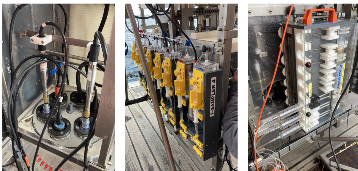
Fig. 5.5 BIGO sensors for measurements of O 2 , conductivity, temperature, H 2 S and STOX (left), fluid sampler for RNA fixation (middle), and additional fluid samplers (right).
